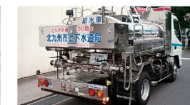
Water tank truck equipped with pump
